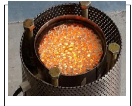
Figure 1: Cordierite based porous burner
